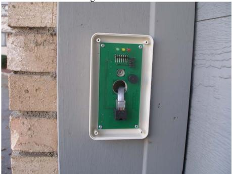
• 6. Re-connect the ribbon cable to the Circuit Board
