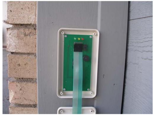
• 7. Carefully replace the Access Keypad Module Cover and the four mounting screws.
