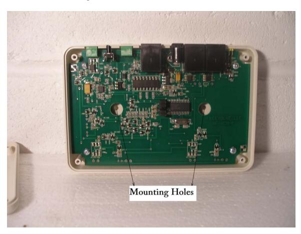
• The Garage Door Controller can be mounted on any accessible location (wall, ceiling, etc). In this example we decided to attach the Garage Door Controller directly to the case of the Garage Door Opener. For this, one of the Garage Door Opener case screws was removed and then re-attached through one of the Garage Door Controller mounting holes:
