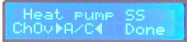
The system sets the active changeover valve state to AC. When finished, navigate to “Done” and press Select. The system will return to the main screen and the Thermostat Module is now configured to work with a single-stage heat-pump HVAC system.
